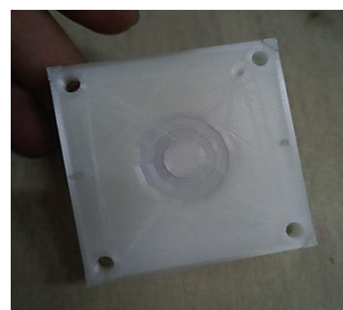
Figure 3. The air pump cover is done
