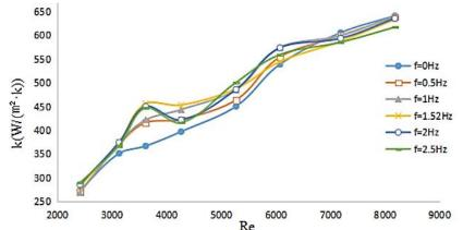
Figure 6. In the case of pulsating flow, the total heat transfer coefficient of the plate heat exchanger at different flow rates
