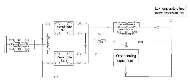
Figure 2. Frequency conversion sea water pump cooling system
