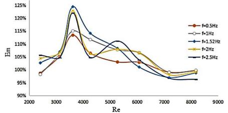
Figure 7. In the case of pulsating flow, the enhanced heat transfer efficiency of the plate heat exchanger at different flow rates
