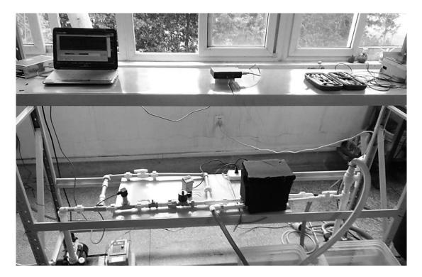
Figure 3. Physical picture of the pulsation enhanced heat transfer experimental system
