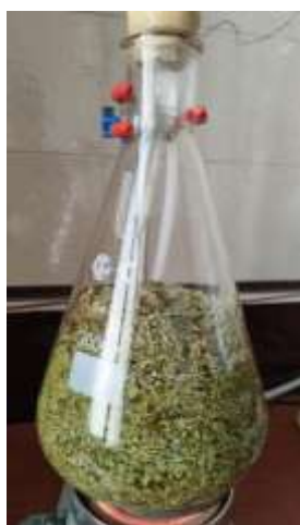
Figure 1. Extraction of essential oil from Thymus vulgaris L.
