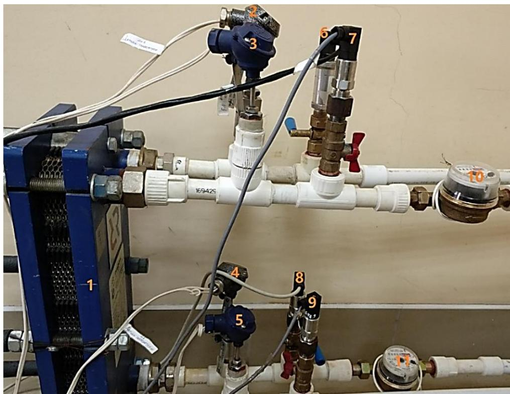
Figure 3. Experimental test section: 1 — plate heat exchanger; 2, 3, 4, 5 — M5100 pressure transmitters; 6, 7, 8, 9 — thermometers; 10, 11 — mechanical flow meters.
