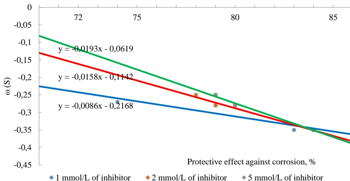
Figure 5. Characteristics of the importance of the charge density on the iron atom (cathodic current density is 4 A / dm<sup>2</sup>).
