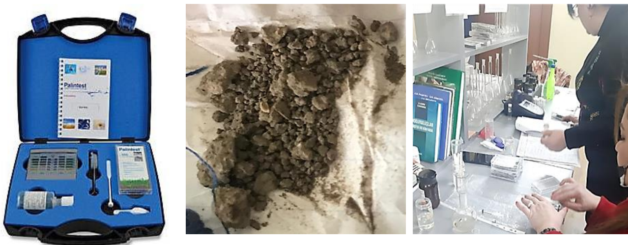
Figure 2. Analysis of soil sample brought from Basitchay State Nature Reserve in the laboratory with Palintest Soil equipment
