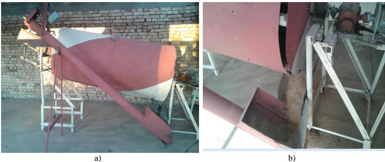
Figure 1. An initial pre-production model of the device for drying of the products of grain crops:
