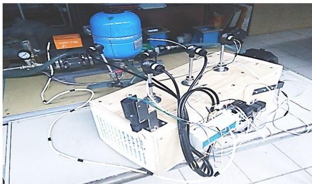
Figure 2. Photo of the exterior of the heat exchanger housing and the complex, including a circulation pump, a hydraulic accumulator, a balancing valve and an electromagnetic fluid flow converter.
