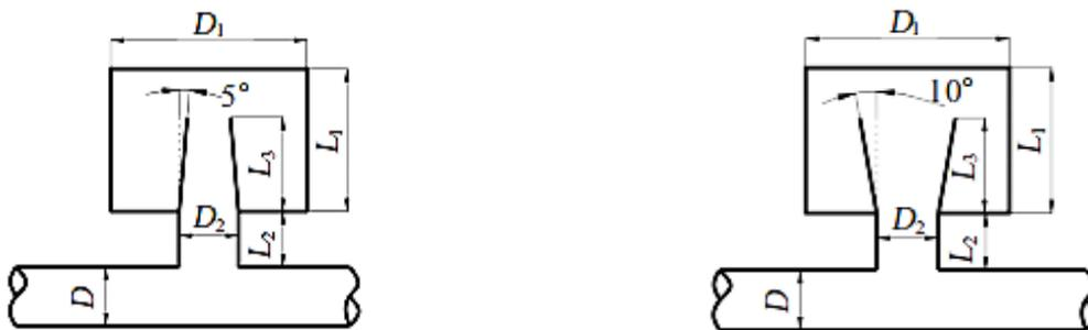
Figure 8. Helmholtz resonator with contraction / expansion extended connecting tube.
